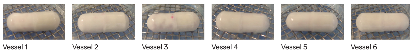
Figure 2: Capsugel® Enprotect® capsules filled with lactose and 0.1% red carrot after 2 hours in HCl 0.1N
